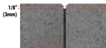
PAVERS OR NATURAL STONES WITH CHAMFER
