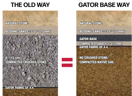
Sand or ASTM No. 9 Stone can be used under stones
