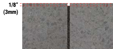
PAVERS OR NATURAL STONES WITHOUT CHAMFER
