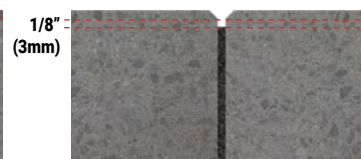
PAVERS OR NATURAL STONES WITH CHAMFER
